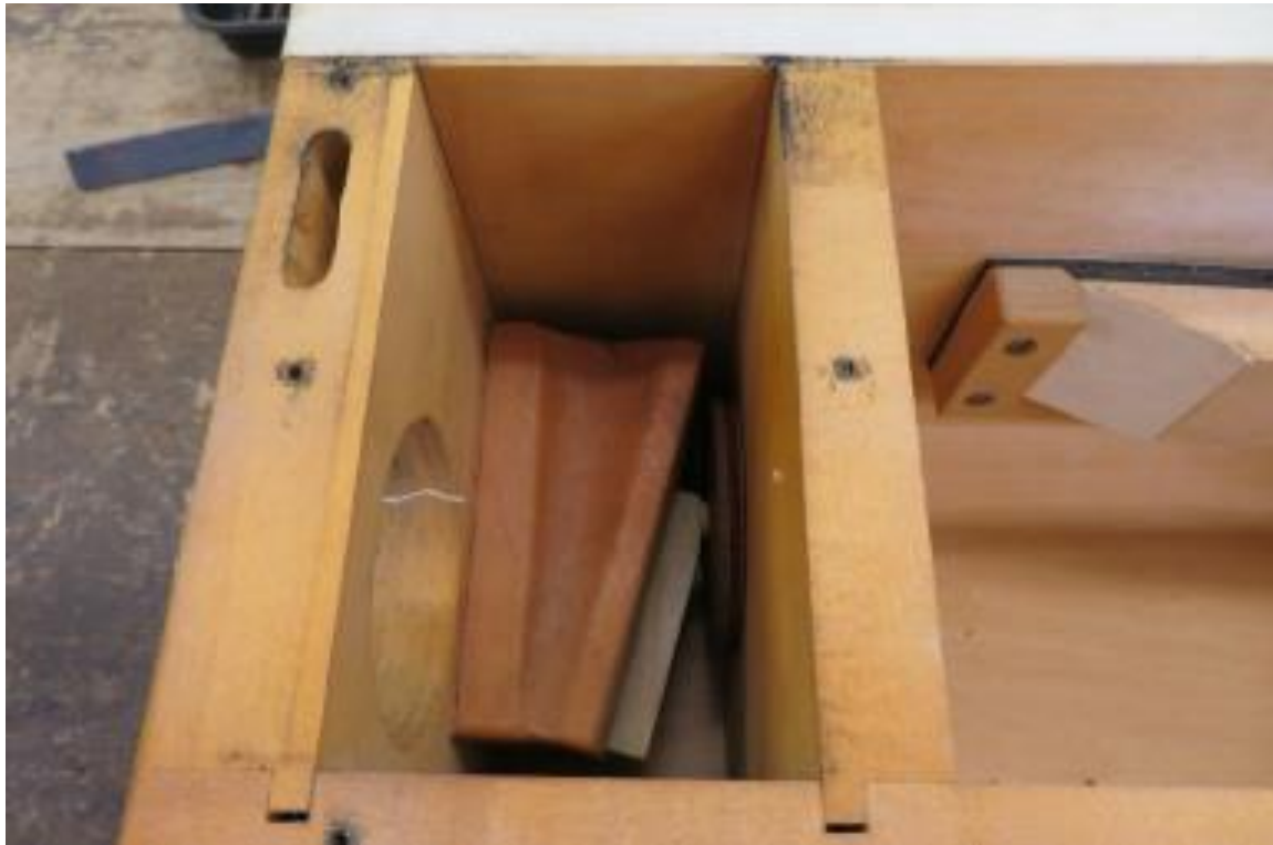
The large stop-action valve inside the Tremolo
