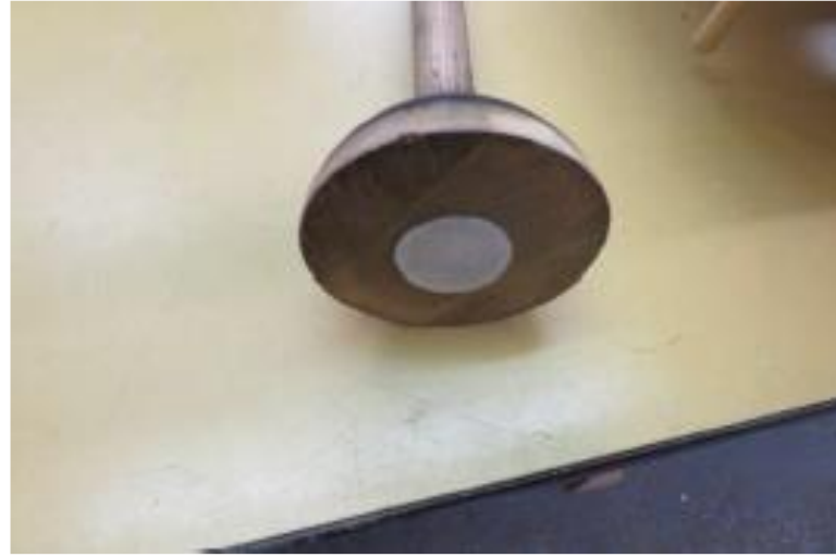
The inside view of the wind-flow regulator valves and the small cone valve
