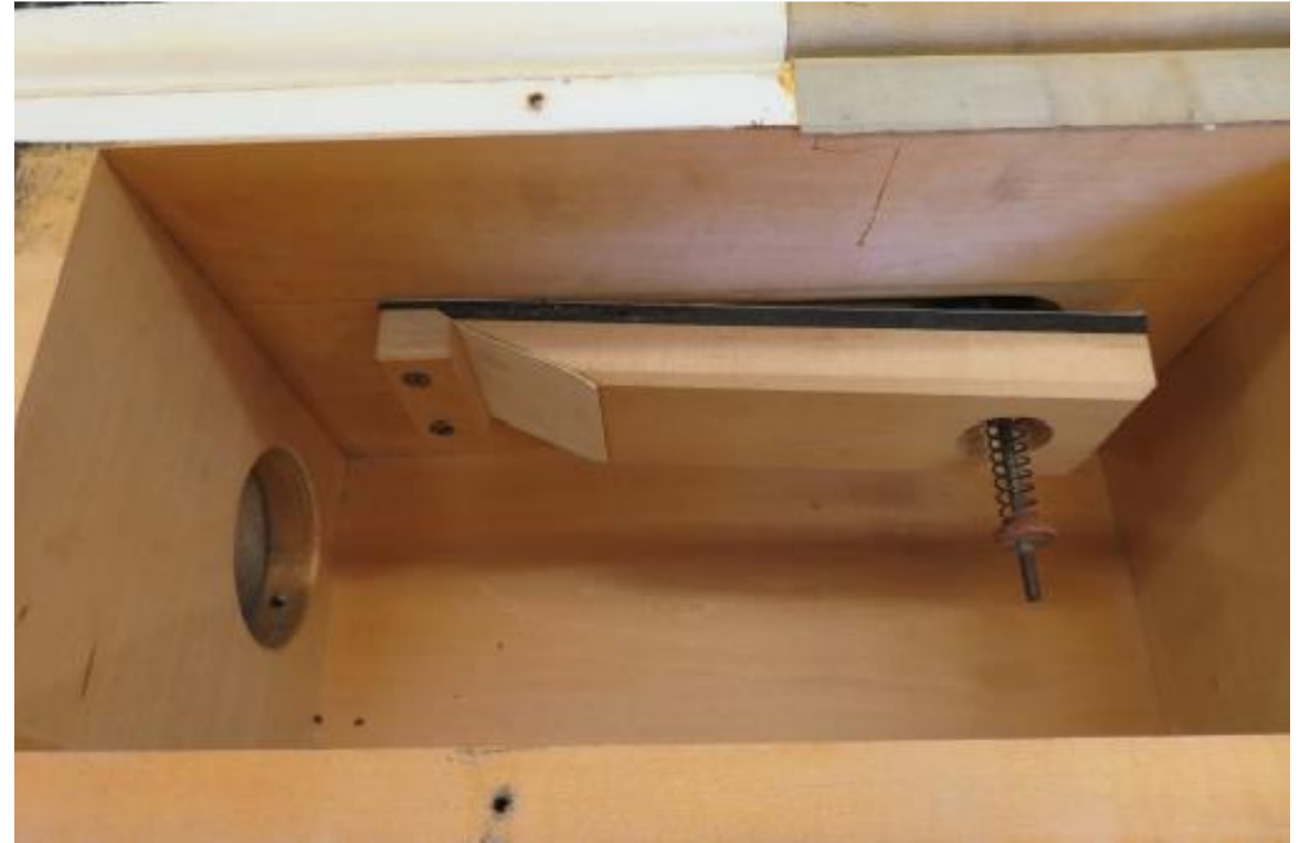
This is the internal pallet valve in one Tremolo machine
