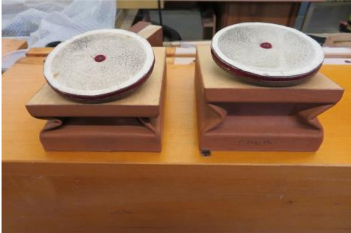
The two large disc valves that work as the stop actions for each of the two Tremolo
