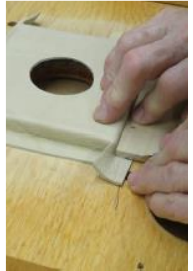
Crafting a new leather seat for the cone-valve
