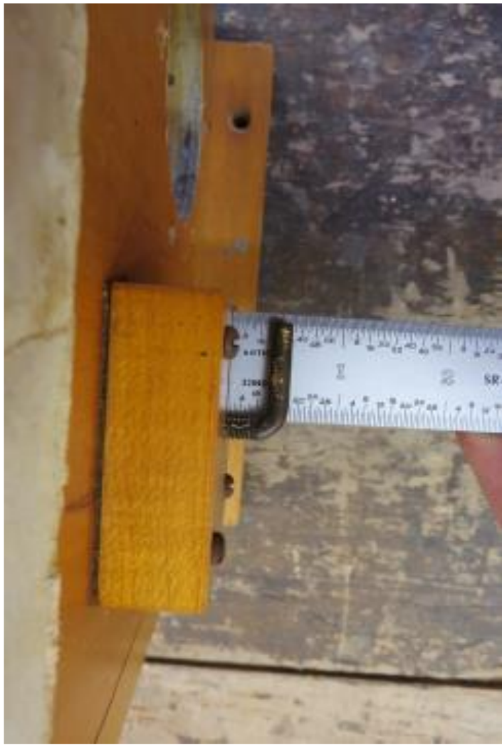
The shop measurement for the depth of the Tremolo effect
